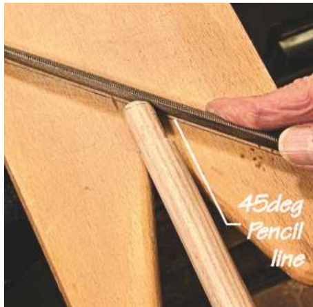
▲ Pic. 6 You can use a V-notched board to locate the arm support and guide the file
